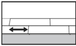
Fig 7. General distances between short ends. Minimum distance between short ends of planks in parallel rows shall not be less than 500 mm. This improves the stability of the floor.
